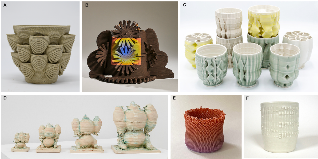
Figure 2: Notable work in the clay 3D printing field that exemplifies common textural and design elements. A) Researcher Sam Bourgault creates mathematically defined cups where the toolpath extends past the vertical edge of the form to create unsupported drooping loops [4]. B) Artist Jolie Ngo prints multiple vertically extruded forms and hand assembles them into complete works [30]. C) Artist Bryan Czibesz creates geometrically evolving surface textures via unique toolpathing [5]. D) Artist Eun-Ha Paek hand builds forms that she scans and re-prints [32]. E) Researcher Leah Beuchley creates irregular surface patterns by excessively increasing the z height between layers [6]. F) Researcher, Audrey Desjardins, and artist, Timea Tihanyi, teamed up to encode audio data in the toolpath of ceramic cups. [10].
